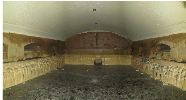
Left: Air-cooling ducts on the outside of a glass furnace. Cooling was lost when power was lost for 9 hours. Right: Inside of glass furnace, said to have been damaged by the loss of cooling.
