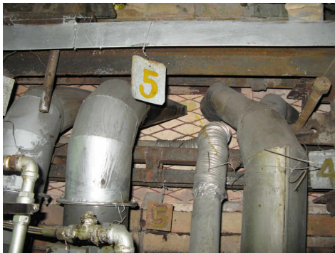
Left: Air-cooling ducts on the outside of a glass furnace. Cooling was lost when power was lost for 9 hours. Right: Inside of glass furnace, said to have been damaged by the loss of cooling.
