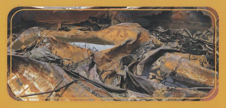
One of a number of newly constructed tanks that exploded. A review of construction records revealed a litany of problems with the internal floating roofs, that remained unresolved when the tanks went into service.
