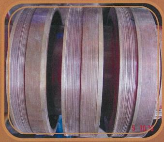
Above is extreme wear on the slip ring of a motor. The motor had been installed in a brick plant where the clay dust had worn the slip ring.
