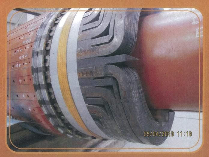
The two pole generator rotor above has suffered overheating and burning of the insulation, as shown by the colours of the insulation and the bare copper. However damage was confined to the rotor, which was able to be rewound at site.
