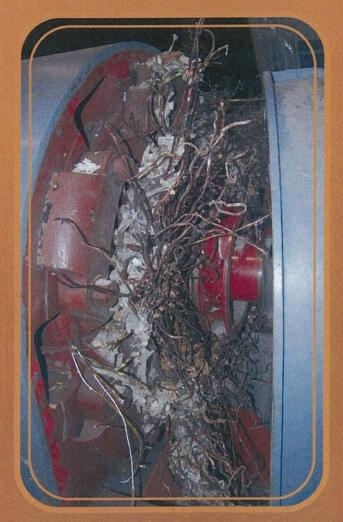
The photograph on the left shows the result of the end ring disintegrating, allowing the overhang of the rotor windings to interfere with the overhang of the stator windings.
